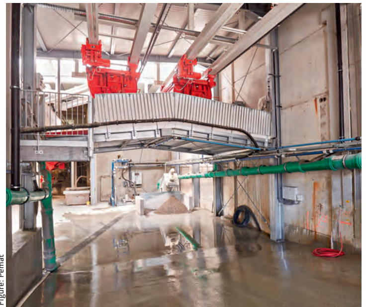
These two mixers are equipped with two discharge doors so that every mixer can feed the material into one of two bucket conveyor systems
