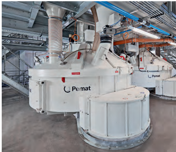
Two Pemat PMPR 3000 planetary mixers with whirler were used, each with a compacted concrete output of 2 cbm
