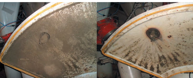
Before and after cleaning with the PHR
