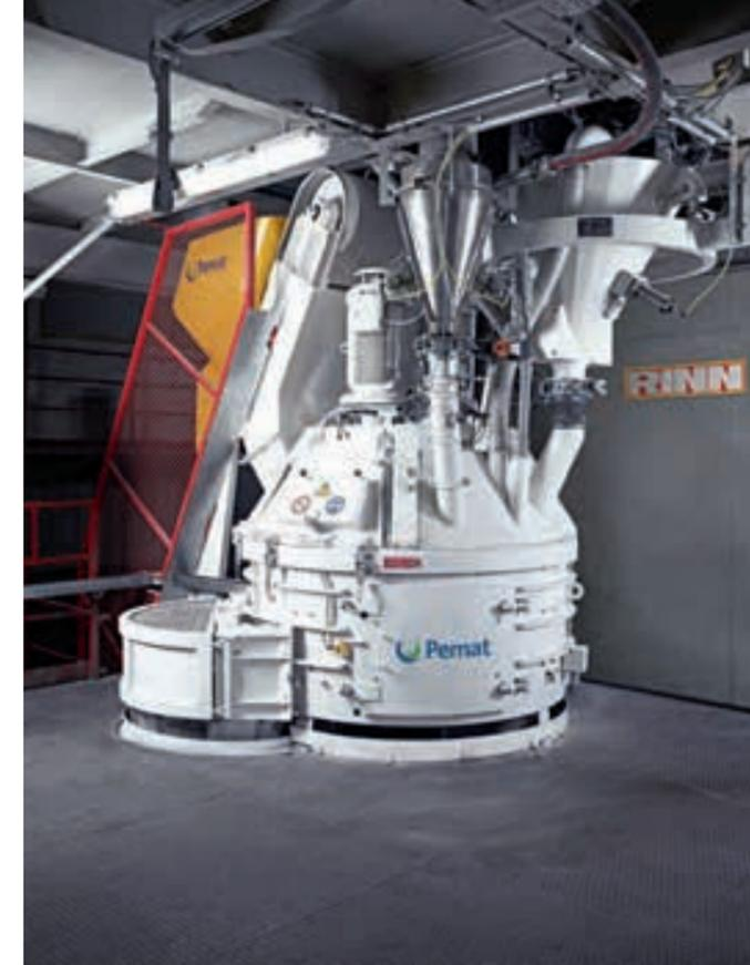
Planetary mixer PMPM 500 Multimix with Skip Hoist PAS
